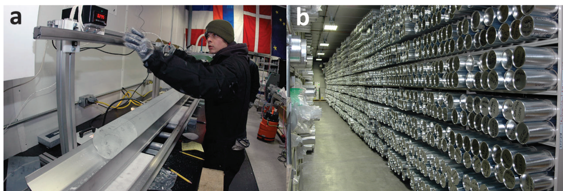
Fig. 14. (a) Measuring an ice core at the 'Unpack' station during one of the NICL CPLs. Photo credit: Peter Rejcek/NSF. (b) View of the inside of the NICL's -36°C archive freezer. Each silver tube on these shelves contains a 1 m long section of the WAIS Divide ice core. Photo credit: Peter Rejcek/NSF.
