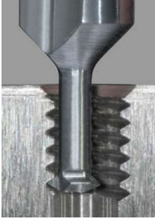
Figure 1. Micro Thread Cutting [6]
