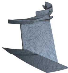
512 513 Figure 12: Turbine mesh for one blade.
