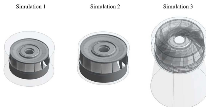
516 517 Figure 13: FEM analysis for the simulations with acoustic fluid.
