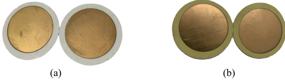
Figure 2. Elaborated samples based flexible PDMS polymer filled with ZnO particles (a) Nano-ZnO/PDMS sample, and (b) Micro-ZnO/PDMS sample.
