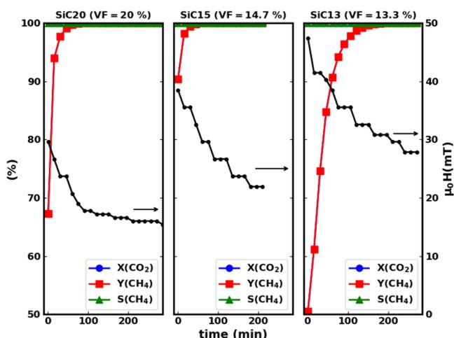
FIG. 9. Catalytic results as a function of time and applied magnetic field  $\mu_0 H$  of samples SiC20, SiC15, and SiC13 [iron mass  $m(\text{Fe}) = 2 \text{ g}$ ]. Since the selectivity is total,  $X(\text{CO}_2)$  and  $Y(\text{CH}_4)$  overlap.
