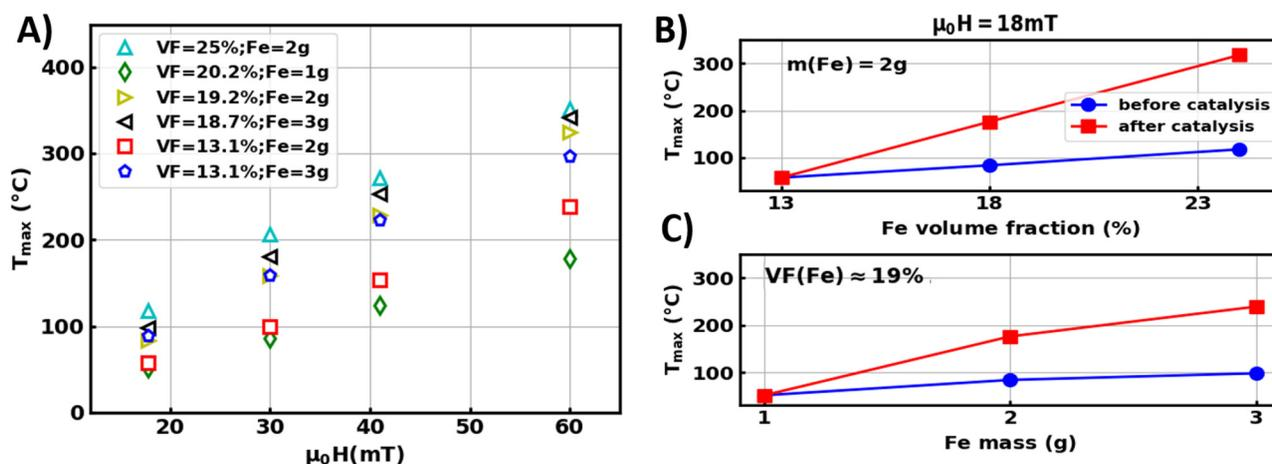
**FIG. 1.** (a) Maximal temperature reached inside the reactor as a function of the applied magnetic field after 10 min. (Right side) Maximum temperature reached inside the reactor under low magnetic field (18 mT) initially and after performing catalysis for more than 2 h. (b) Different iron volume ratios and constant Fe mass [ $m(Fe) = 2g$ ]. (c) Constant iron volume ratio ( $VF \approx 19\%$ ) and varying Fe masses.
