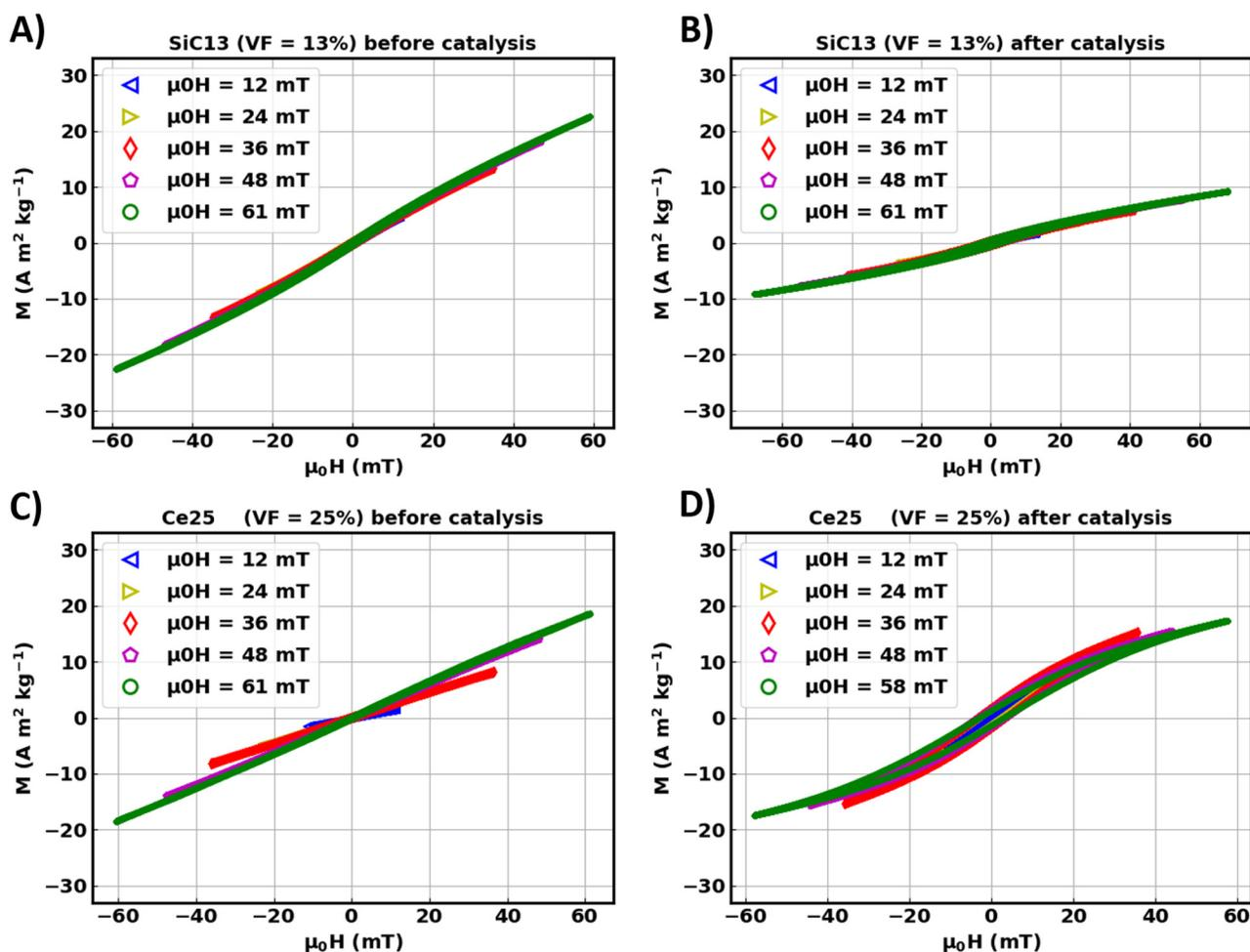
FIG. 5. Hysteresis cycles at room temperature and 50.33 kHz. Sample SiC13 (a) initially and (b) after catalysis. Sample Ce25 (c) initially and (d) after catalysis.
