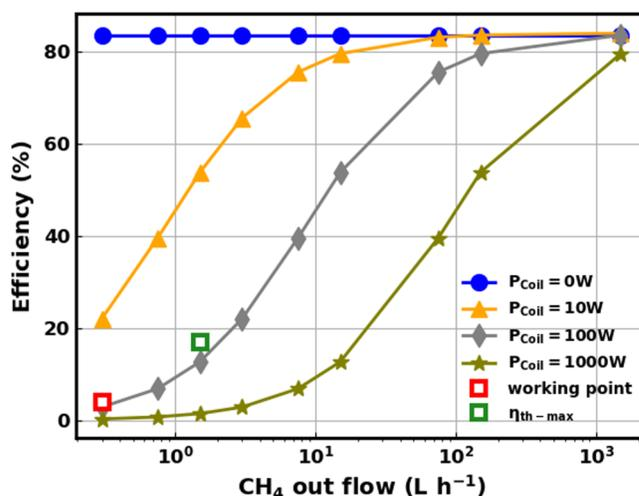
FIG. 11. Sabatier reaction efficiency calculated from Eq. (2) as a function of  $\text{CH}_4$  outflow (with 100% yield) for different input coil's power. The current working efficiency (flow =  $0.3 \text{ l h}^{-1}$ ,  $P_{\text{coil}} = 70 \text{ W}$ , red square) and the maximum theoretical efficiency of our setup (green square) are also indicated.
