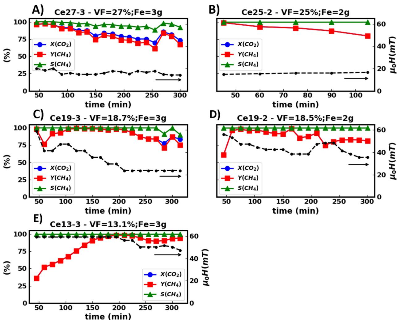
FIG. 8. Catalytic performance (plain lines) and applied magnetic field  $\mu_0 H$  (black dash-dotted line) vs time for different iron volume fractions and masses of SiC-free catalysts. Whenever the selectivity  $S(\text{CH}_4)$  is total, the conversion  $X(\text{CO}_2)$  and the yield  $Y(\text{CH}_4)$  overlap.
