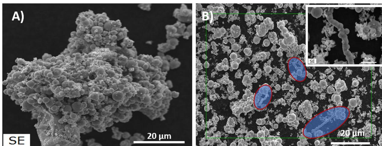
**FIG. 3.** SEM image after magnetic field exposure in the standard conditions: (a) Fe/Ni/CeO<sub>2</sub> catalyst (sample Ce25-2, VF = 25%) and (b) Fe/Ni/CeO<sub>2</sub>/SiC catalyst (sample SiC13). The inset shows a zoom in on a chain from a different location in the sample.
