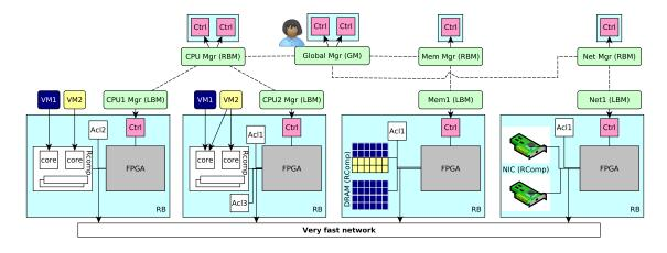
Figure 2. The NewVirt platform for rack-scale disaggregated virtualization.
