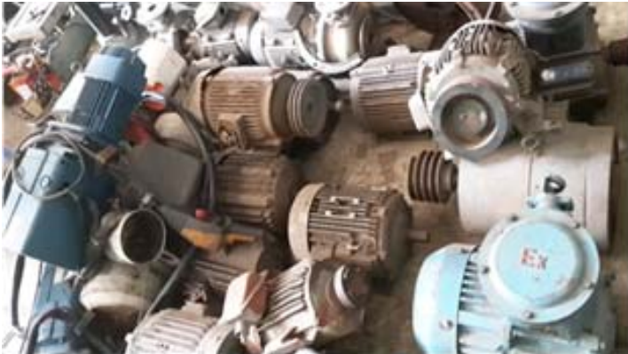
Fig. 2: Induction recovery motors in Cambodia (low cost second hand products from China, Taiwan, Malaysia, Thailand...)
