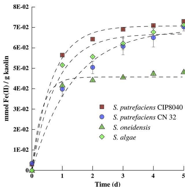
**Fig. 1.** Iron leaching from kaolin using various iron-reducing bacteria at 20 °C. All experiments were run with 20 g of kaolin and  $(1.05 \pm 0.35) \times 10^7$  CFU mL<sup>-1</sup> of cell suspension. The initial rate of reduction was computed from the first derivation of a nonlinear curve fit represented by the dotted lines. Errors bars represent standard deviation of three triplicates incubations.
