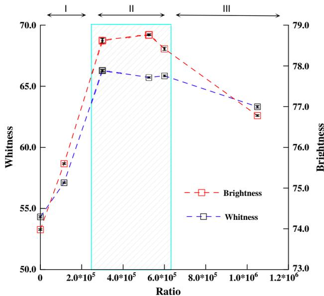
**Fig. 3.** Whiteness and brightness evolution after 5 days of incubation as the function of cell/kaolin ratio (CFU/g kaolin). The blue box represents the best cell/kaolin ratio identified in this study, to achieve a noticeable improvement of the kaolin colour properties. The error bars represent standard deviation of six separate analyses.
