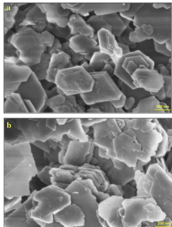
Fig. 6. SEM micrographs of kaolin before and after its bioleaching for 5 days by *S. putrefaciens* CIP8040 at 30 °C using 20 g of clay. (a) represents the untreated kaolin, and (b) the bioleached kaolin.
