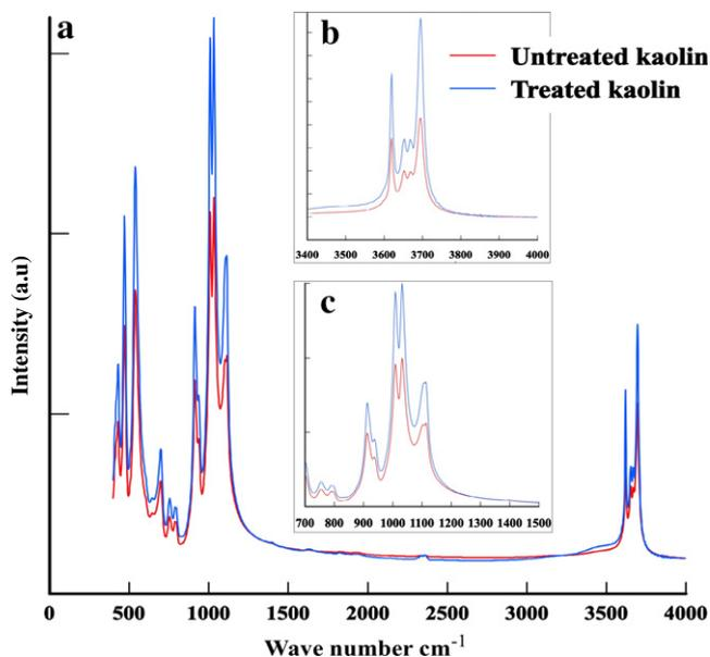
Fig. 5. FTIR spectra of the kaolin before and after its bioleaching for 5 days by *S. putrefaciens* CIP8040 at 30 °C using 20 g of clay. Inset (b) represents the region of OH stretching and (c) the region of structural vibration.
