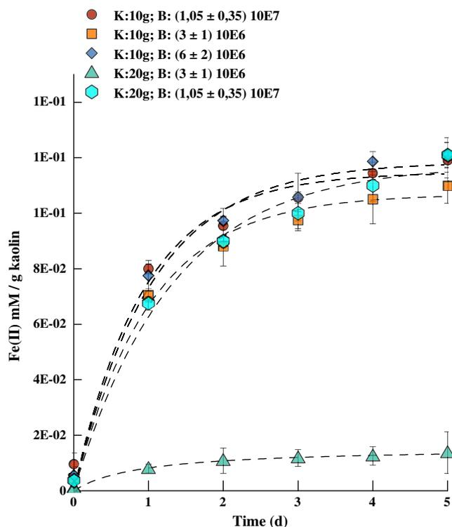
Fig. 2. Fe bioleaching of 10 and 20 g of kaolin at  $30 \text{ }^\circ\text{C}$  with different cell concentrations. The initial rate of reduction was computed from the first derivation of a nonlinear curve fit represented by the dotted lines. Errors bars represent standard deviation of triplicates batches incubations.
