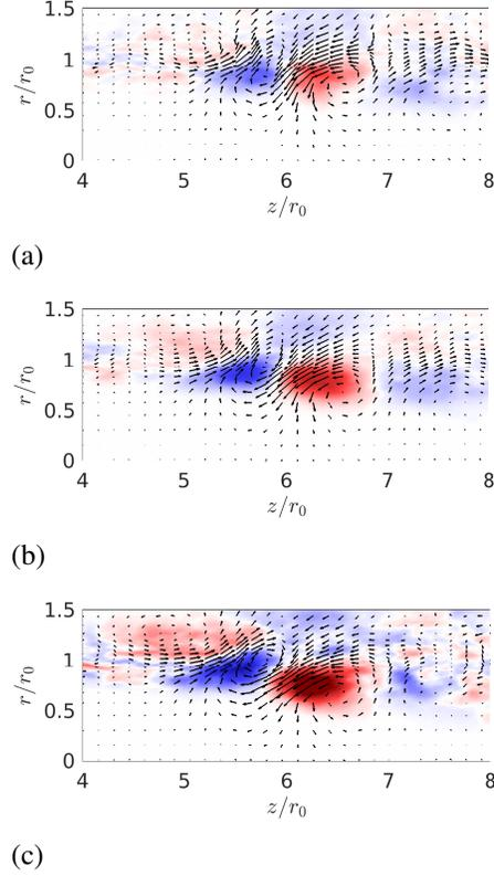
**Fig. 11** Representation at  $t = t_s$  of the conditional velocity as a vector field with the vorticity in color scale for (a)  $p_{max} < 2.5p_{rms}$ , (b)  $3p_{rms} < p_{max} \leq 3.5p_{rms}$  and (c)  $p_{max} \geq 4p_{rms}$ . The scale for the vorticity ranges between  $\pm 2u_j/r_0$
