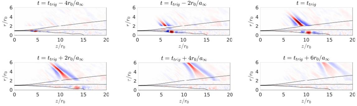
**Fig. 7 Representation of conditional pressure fluctuations outside the jet and of conditional vorticity norm inside. The scales range between  $\pm 5,000$  Pa for the pressure and  $\pm u_j/r_0$  for the vorticity. The solid lines indicate contours of conditional axial velocity for the values  $0.95u_j$ ,  $a_\infty = 0.5u_j$  and  $0.05u_j$ .**
