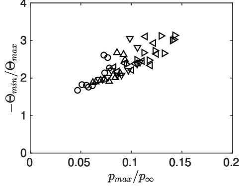
**Fig. 6** Conditional steepening factor as a function of the conditional pressure peak for  $6r_0 \leq z_{trig} \leq 15r_0$  and  $\circ p_{max} < 2.5p_{rms}$ ,  $\triangle 2.5p_{rms} \leq p_{max} < 3p_{rms}$ ,  $\nabla 3p_{rms} \leq p_{max} < 3.5p_{rms}$ ,  $\triangleleft 3.5p_{rms} \leq p_{max} < 4p_{rms}$  and  $\triangleright p_{max} \geq 4p_{rms}$
