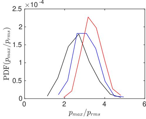
**Fig. 4** PDF of the pressure peaks at  $z = 8r_0$  and  $r = 2.8r_0$  for interval length  $\tau$  of  $\text{---}$   $0.5r_0/a_\infty$ ,  $\text{---}$   $r_0/a_\infty$  and  $\text{---}$   $2r_0/a_\infty$
