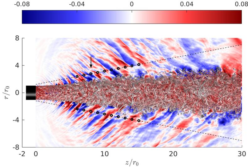
**Fig. 1** Positive isosurface of  $q$ -criterion  $q = 0.65(u_j/r_0)^2$  colored by the jet velocity and pressure fluctuations  $p'/p_\infty$  outside the jet. The circles represent the detection positions for the conditional averages and the arrow indicates the location of peak pressure levels on the cylindrical surface.
