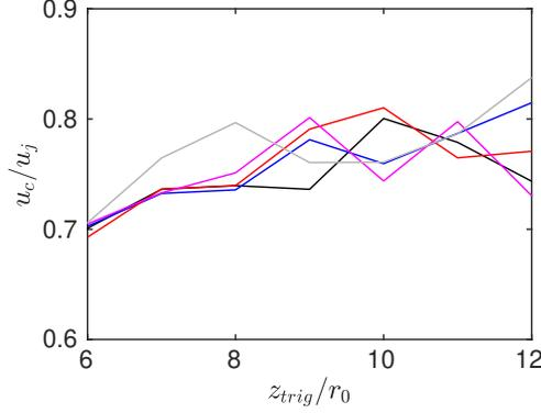
**Fig. 8** Axial variations of the convection speed for  $p_{max} < 2.5p_{rms}$ ,  $2.5p_{rms} \leq p_{max} < 3p_{rms}$ ,  $3p_{rms} \leq p_{max} < 3.5p_{rms}$ ,  $3.5p_{rms} \leq p_{max} < 4p_{rms}$  and  $p_{max} \geq 4p_{rms}$
