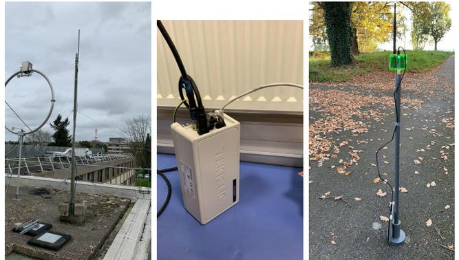
(a) Position of the gateway monopole antenna fixed on the roof. (b) The gateway device connected to the antenna and connected to a battery at location 7. (c) The packaged Pycom device fixed on a rod.
