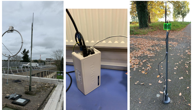
(a) Position of the gateway monopole antenna fixed on a roof. (b) The gateway device connected to the antenna and connected to a battery at location 7. (c) The packaged Pycom device fixed on a pole.
