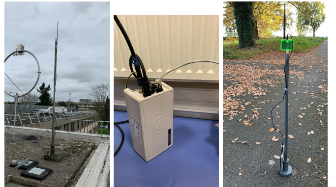
(a) Position of the gateway monopole antenna fixed on a roof. (b) The gateway component connected to the antenna rod and connected to a battery at location 7. (c) The packaged Pycom device fixed to a battery at location 7.
