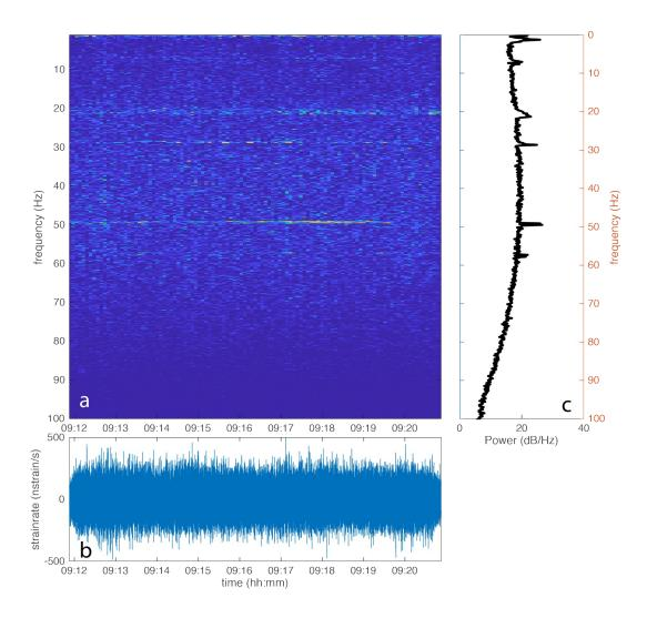
**Figure 3** Strain-rate measured on the optical fiber at a distance of 20km from the shore while the tanker was passing above the cable and shown by the power spectrogram between 0 and 100Hz (a), the corresponding time series (b) and the average power spectral density for 9 minutes time records(c).
