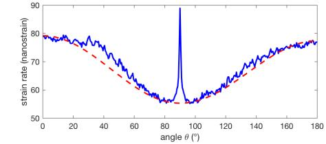
Figure 10 Beamforming output for (blue line) linear depth DAS-array between 4600-5912m off the coast, corresponding to a depth ranging from 100 to 200m, assuming a velocity of 1530m/s. The dashed line shows the cos2 broadside sensitivity for acoustic waves.
