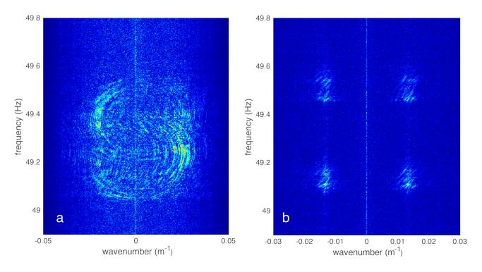
Figure 8 Frequency-wavenumber (f-k) decomposition of 8 minute long strain-rate signal between 48.9 and 50.1 Hz, for seaward (k<0) and landward (k>0) components and for the 4.5-7.5km and the 17-22km sections of the fiber (a) and (a) respectively when the tanker passed over the cable
