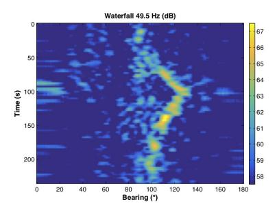
**Figure 11** Beamforming performed over a linear antenna of 256m length and centered at 5741m from the fiber extremity. Focalization is around 550m. The beamforming is performed every 5 seconds using the recorded signal filtered in the [48 51]Hz band.
