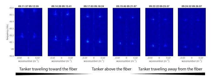
**Figure 9** Frequency-wavenumber (f-k) decomposition of the strain-rate windowed on 1.3 minutes long signal between 48.9 and 49.6 Hz, for seaward (k<0) and landward (k>0) components for the the 17-22km sections of the fiber when the tanker passed 2000m above the cable.
