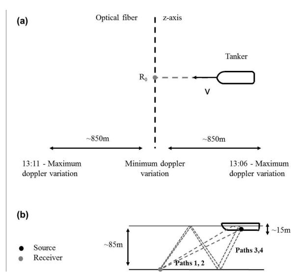
Figure 4 Ship displacement (a) top view (b) side view
