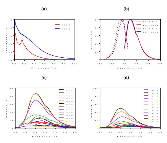
**Figure 3:** (a) UV-vis spectra of CQD-1 and CQD-2 at 20 μg mL<sup>-1</sup> in PBS (pH 7.4, 0.01 M). (b) Normalized emission (exc. at 378 nm) and normalized excitation (em. 453 nm) spectra of CDQ-1; normalized emission (exc. at 382 nm) and normalized excitation (em. 452 nm) spectra of CQD-2. (c) Emission spectra of CQD-1 at progressively increasing excitation wavelengths from 280 to 500 nm. (d) Emission spectra of CQD-2 at progressively increasing excitation wavelengths from 280 to 500 nm.
