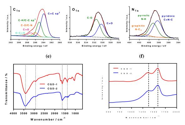
**Figure 2:** (a) Schematic representation of the synthesis of CQD-1 and CQD-2. (b) AFM images of CQD-1 and CQD-2 together with size distribution histograms. (c) XPS analysis of CQD-1:  $C_{1s}$ ,  $O_{1s}$  and  $N_{1s}$ . (d) XPS analysis of CQD-2:  $C_{1s}$ ,  $O_{1s}$  and  $N_{1s}$ . (e) FT-IR spectra of CQD-1 (red) and CQD-2 (blue). (f) Raman spectra of CQD-1 (red) and CQDs-2 (blue).
