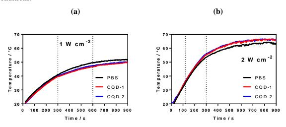
**Figure 4: Photothermal properties of CQDs.** Temperature profiles of CQDs (50 μg mL<sup>-1</sup>) upon laser irradiation at 810 nm laser at two different power densities: 1 W cm<sup>-2</sup> (a) and 2 W cm<sup>-2</sup> (b).
