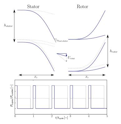
Figure 5: Design recommendation for a turbine driven by a pulsed flow. Recommendations are identified by lines (---). The lines (---) show the experimental domain. It should be noted that the speed triangle shown is a pictorial, albeit very inadequate, way of characterizing the rotor speed in relation to a semblance of flow speed.
