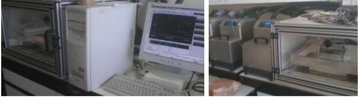
Figure 5- Thermal characterization device for building materials
