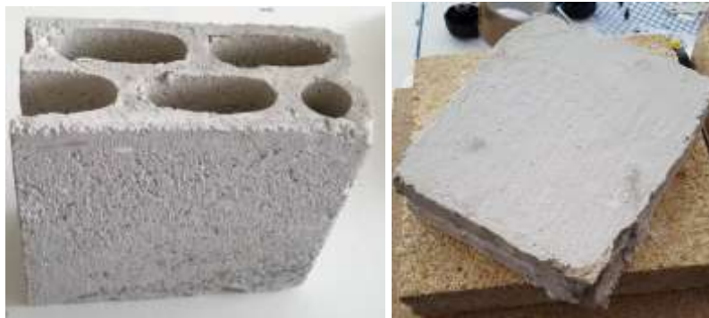
Figure 4- Experimented samples of the hollow block (left) and the solid mixture (right)
