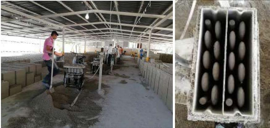
**Figure 2- Work area of the craftsman and mold**
