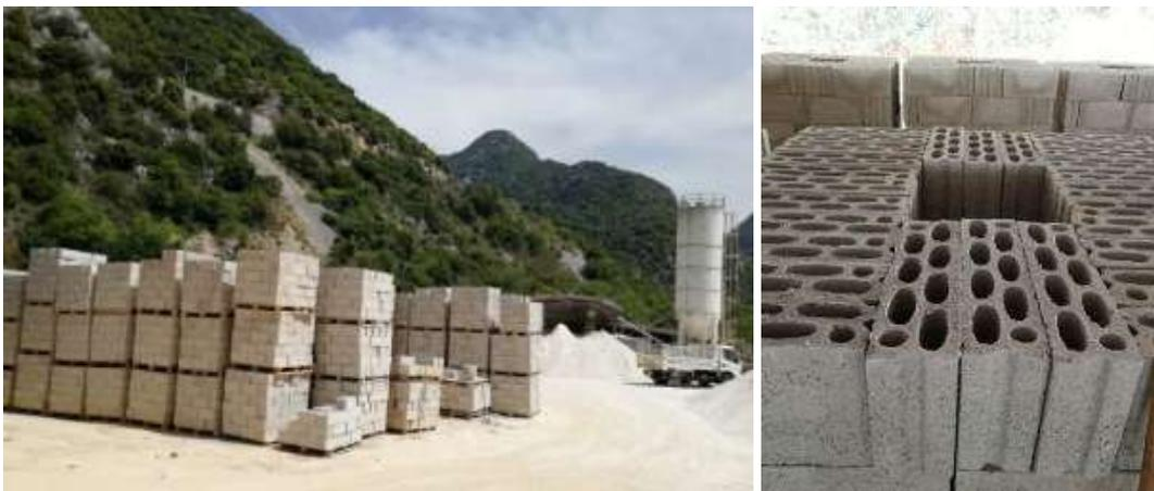
**Figure 3- Storage and drying of the blocks**
