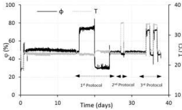
**Figure 6- Static solicitation of relative humidity and temperature**
