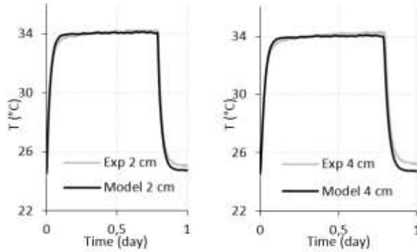
**Figure 12- Measured and modelled temperature evolution at  $x = 2$  cm and  $4$  cm respectively (2<sup>nd</sup> protocol)**
