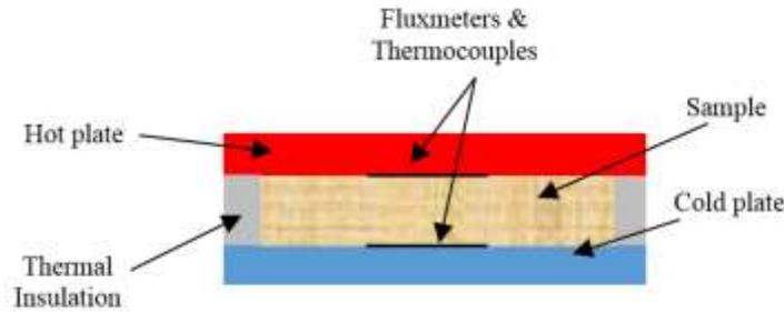
**Figure 3- Schematic of principle heat flow meter method**
