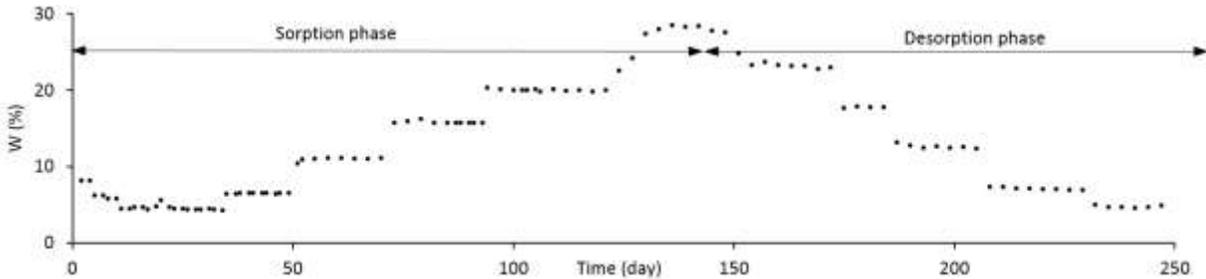
**Figure 1- Kinetic sorption isotherm of wood fiber**
