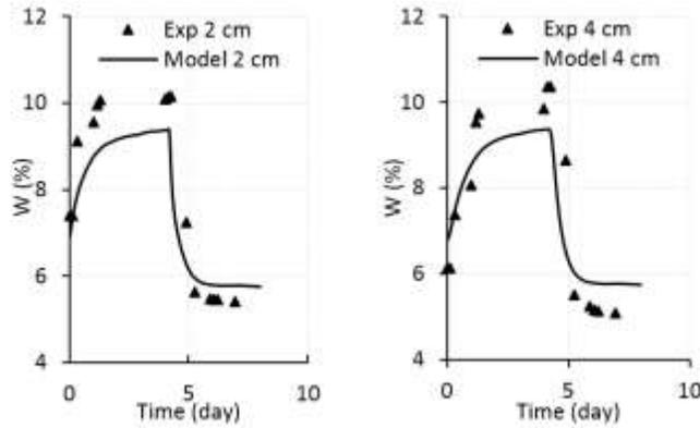
**Figure 11- Measured and modelled Water content evolution at  $x = 2$  and  $4$  cm (1<sup>st</sup> protocol)**
