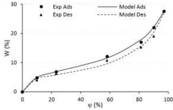
**Figure 2- Adsorption and Desorption curve of wood fiber**
