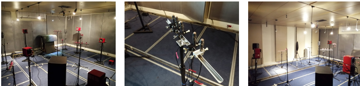
Figure 2: Pictures of the acoustic lab. From left to right: the overall setup, one microphone array, the setup with revolved panels.
