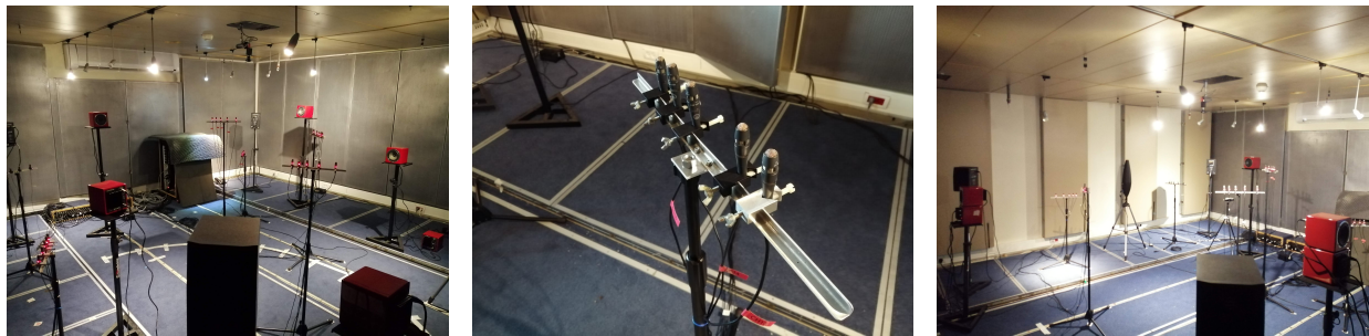
Figure 4 Picture of the acoustic lab. From left to right: the overall setup, one microphone array, the setup with revolved panels.
