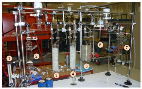
Figure 1 Photograph of the DIC extraction line. 1: the flowmeter; 2: stripping vessel; 3, 4, 5: cold traps (respectively at 80, 80, and 190 °C); 6: cold finger with a MKS gauge; 7: 2 aliquots in 2 different vials. Vacuumis generated by a dry primary pump coupled to a turbopump. Residual pressure is measured by 2 full range Pfeiffer gauges.
