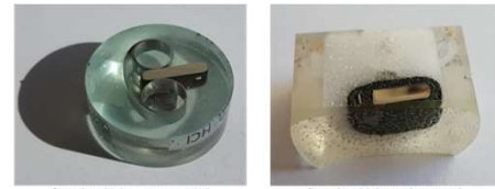
Sample which was suspended Sample which was immersed Macrophotos of the two types of samples being metallographically prepared
