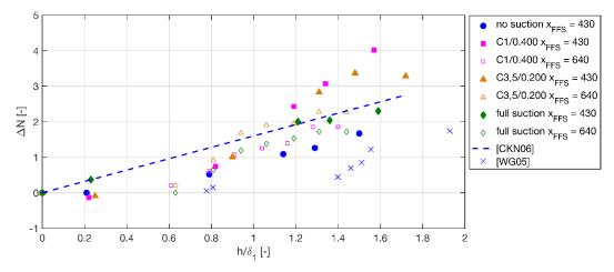
Figure 7. All suction configurations with FFS compared with  $\Delta N$  model from [15] and with experimental data from [14].
