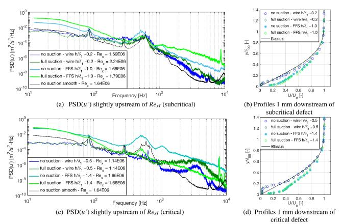
Figure 6. Spectral analysis of the velocity fluctuations just upstream of transition location and boundary-layer profiles just downstream of the defects (wires and FFS)
