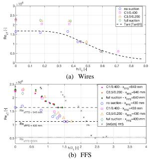
Figure 4. Transition Reynolds number as a function of  $h/\delta_1$  for wires and FFS.
