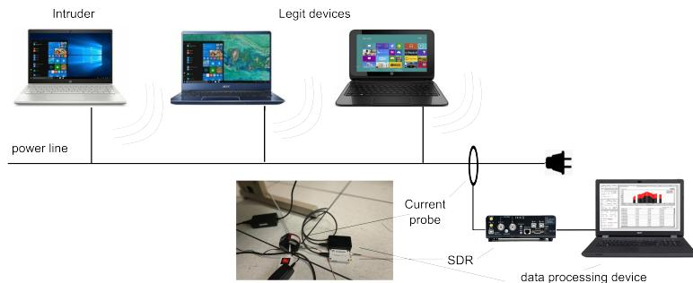
**Fig. 1.** Block diagram of the proposed method: the network is made of legit devices and an intruder. All generate EM emanations that couple onto the power lines. The proposed method captures the EM signal with a current probe and SDR system that sends the raw IQ data to a processing data device.
