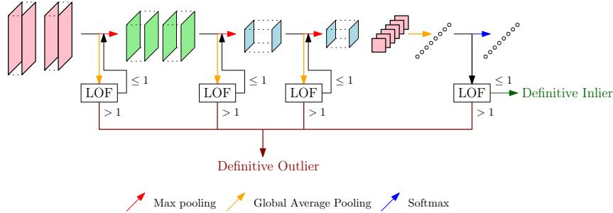
**Fig. 4.** Presentation of the CLOF anomaly detection module.
