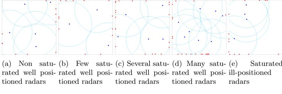
Fig. 1: The 5 validation scenarios (radars &amp; FOV in blue, targets in red)
