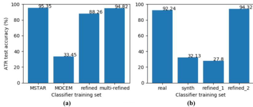
**Fig. 6.** Accuracy of ATR classifiers trained with (a) MSTAR/MOCEM, (b) SAMPLE
