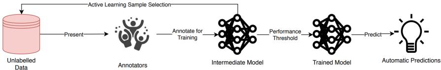
**Fig. 1. Schematics of the active learning iterative process (from [3]).**
