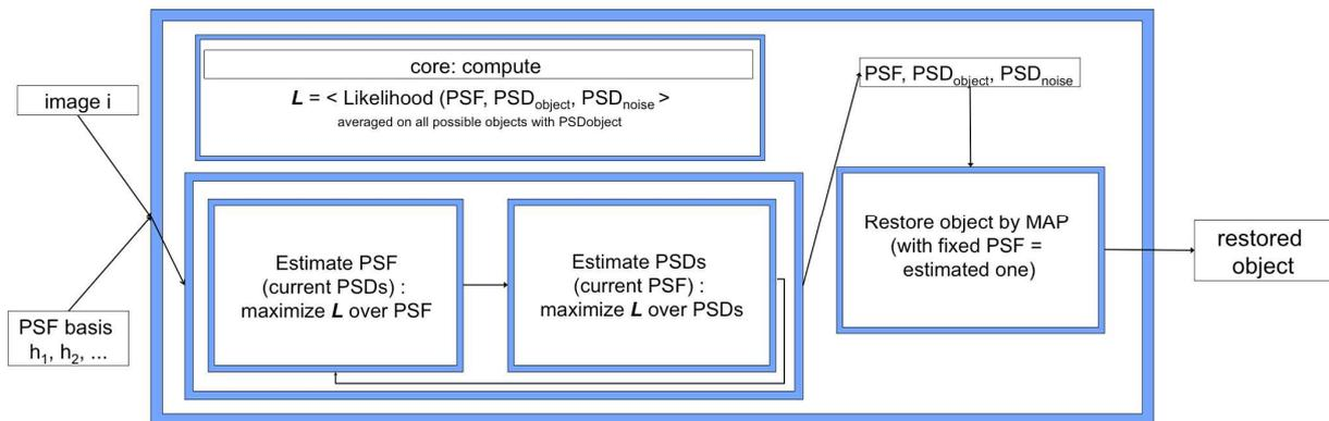
**Fig. 4** Sketch of the deconvolution procedure.
