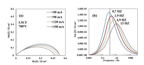
Fig. S4. Experimental and simulated impedance diagrams for the LSCF electrode at 700°C under air for  $i_{dc} = +50$ , +90, +120 and +150 mA·cm<sup>-2</sup> (a) and (b) Nyquist and Bode plots.
