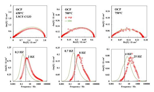
Fig. S2. Experimental and simulated impedance diagrams at OCP for the LSCF-CGO electrode. Nyquist plots for (a) 650°C, (b) 700°C and (c) 750°C – Bode plots for (d) 650°C, (e) 700°C and (f) 750°C.
