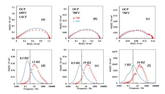
Fig. 5. Experimental and simulated impedance diagrams for the LSCF electrode at OCP. Nyquist plots for (a) 650°C, (b) 700°C and (c) 750°C. Bode plots for (d) 650°C, (e) 700°C and (f) 750°C.
