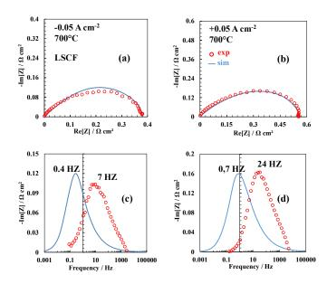
Fig. 6. Experimental and simulated impedance diagrams for the LSCF electrode at 700°C for  $i_{dc} = \pm 50$  mA cm<sup>-2</sup>. (a) and (b) Nyquist and (c) and (d) Bode plots.
