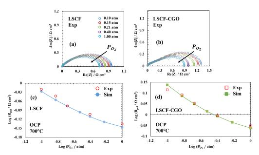
Fig. 7. Nyquist plots as a function of the oxygen partial pressure at 700°C for (a) the LSCF and (b) the LSCF-CGO electrode, respectively. Plot of the logarithm of the electrode polarization resistance as a function of the logarithm of the oxygen partial pressure for (c) the LSCF electrode and (d) the LSCF-CGO electrode.
