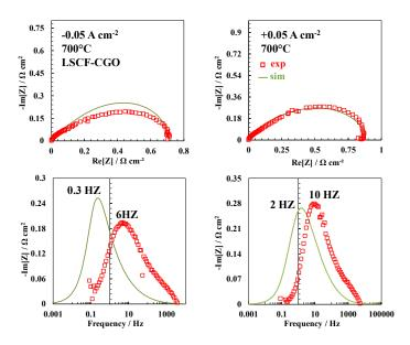
Fig. S3. Experimental and simulated impedance diagrams for the LSCF-CGO electrode at  $700^{\circ}$ C for  $i_{dc} = \pm 50 \text{ mA} \cdot \text{cm}^{-2}$  (a) and (b) Nyquist and (c) and (d) Bode plots.
