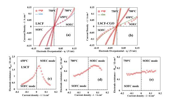
Fig. 4. Experimental and simulated experimental i-η curves under air for (a) the LSCF and (b) the LSCF-CGO electrode [32], respectively. Experimental LSCF electrode polarization resistance plotted as a function of the current density at (c) 650°C, (d) 700°C and (e) 750°C.
