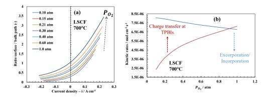
Fig. 9. (a) Ratio of the surface/bulk path as a function of the current density for each investigated oxygen partial pressure at  $700^{\circ}$ C for the LSCF electrode. (b) Kinetic rates of the oxygen excorporation/incorporation (blue) and the charge transfer at TPBIs (red) as a function of the oxygen partial pressure computed close to the OCP (at +0.225 mA·m<sup>-2</sup>).
