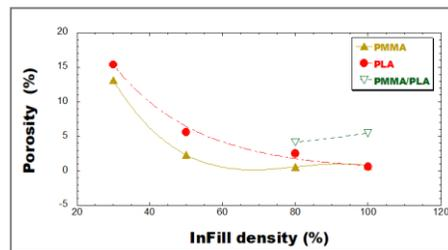
Fig. 7. Porosity percentage versus infill density.
