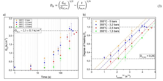
Fig. 3. (a) Evolution of the mode I interlaminar fracture toughness versus contact time for different contact pressure at 355°C and (b) the corresponding healing degree. The linear fit correspond to the identification of the healing kinetics.
