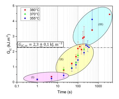
Fig. 2. Evolution of interlaminar fracture toughness for three isothermal temperatures versus contact time. Highlight of the three identified bonding regimes
