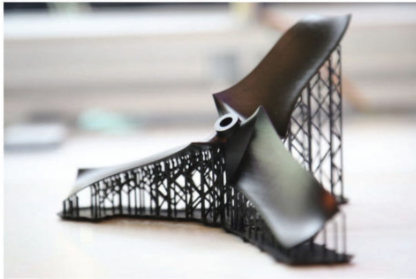
Figure 1. Optimized rotor, 3D printed with SLA technology. Sources: Usine Nouvelle [copyright].
