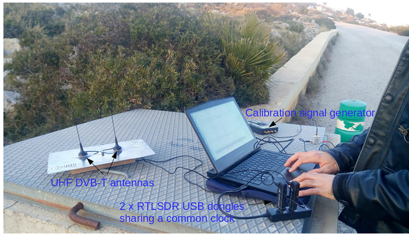
FIGURE 13 Ultra low cost antenna array prototype with N = 2 elements [Color figure can be viewed at wileyonlinelibrary.com and www.ion.org ]
