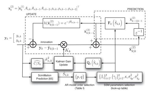
Fig. 5. Block diagram of the new adaptive EKF-based architecture.
