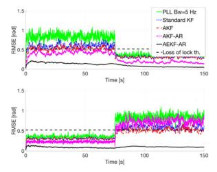
Fig. 9. RMSE considering time-varying scintillation conditions. Severe  $(S_4 = 0.8 \text{ and } \tau_0 = 0.2)$  to moderate  $(S_4 = 0.5 \text{ and } \tau_0 = 0.4)$  scintillation transition (top) and vice versa (bottom).
