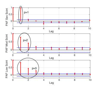
Fig. 14. Sample PAF for real scintillation data model order selection. Severe (top), moderate (middle), and low (bottom) real phase scintillation.
