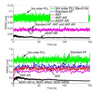
Fig. 6. (Top) RMSE obtained with the proposed AEKF-AR and the SoTA techniques for a scintillation-free standard scenario. (Bottom) RMSE obtained with different methods specified in Table II for a severe scintillation ( $S_4 = 0.8$  and  $\tau_0 = 0.2$ ) propagation scenario.
