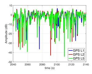
Fig. 10. An example of 100 s of real scintillation amplitude data for the strong scintillation event #1 at three different GPS frequency bands.
