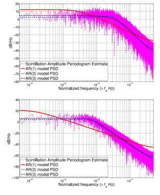
Fig. 1. Scintillation amplitude CSM time-series AR(q) approximation example. Severe (top)  $\{S_4 = 0.9, \tau_0 = 0.1\}$  and moderate (bottom)  $\{S_4 = 0.5, \tau_0 = 0.4\}$  scintillation amplitude cases.
