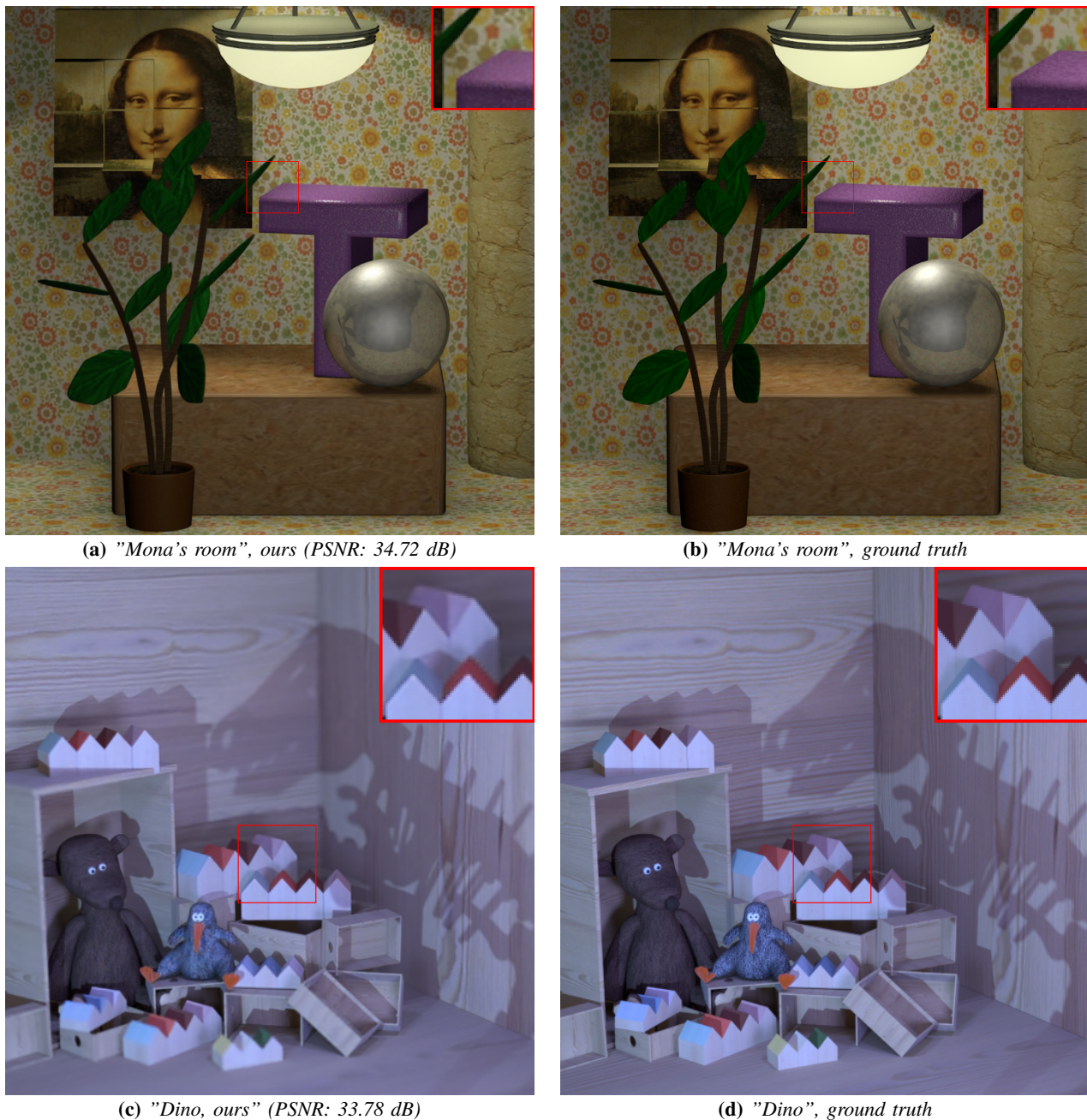
Fig. 11: Reconstructed central view of the Mona's Room and Dino light fields from the HCI dataset [39] using the proposed pipeline with Bayer CFA and learned CCM architecture.
