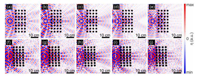
FIG. S2: Valley-Hall edge states: Experiments, and simulations. The water surface is perforated by  $4 \times 8$  square rigid inclusions. Numerics (top) and experiments (bottom) are shown at frequencies (a, f) 6.7 Hz, (b, g) 7 Hz, (c, h) 7.3 Hz, (d, i) 7.6 Hz and (e, j) 7.9 Hz.
