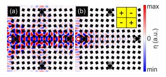
FIG. 5: Numerical illustration for a three-way splitter at 7.3 Hz: Four quadrants of alternately squares rotated clockwise and counter-clockwise. The valley-Hall phases, associated with the propagating modes, are shown within the yellow inset. (a) has no losses whilst (b) incorporates attenuation introduced by considering a complex wave velocity with 2% imaginary part relative to the real part.
