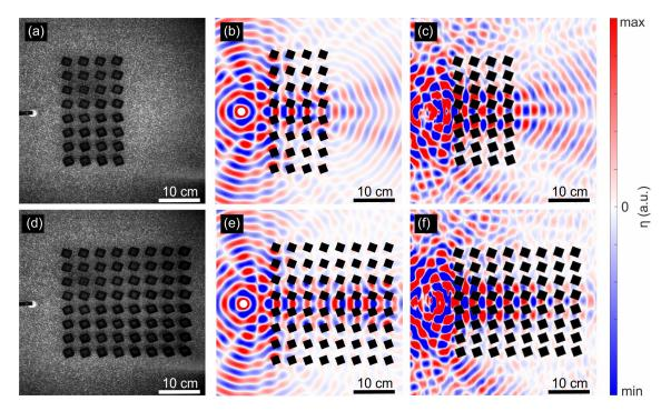
FIG. 4: Valley-Hall edge states: Experiments, and simulations. (a,d) Experimental set-up showing the top view of the water surface perforated by 4 × 8 and 8 × 8 square rigid inclusions respectively. (b,e) Corresponding numerical calculations; (c,f) Experimentally observed wavepatterns. These valley-Hall states are generated by a monopolar source operating at a frequency of 7.3 Hz and placed 6 cm from the domain wall edge and propagate between inclusions rotated by ±20°.
