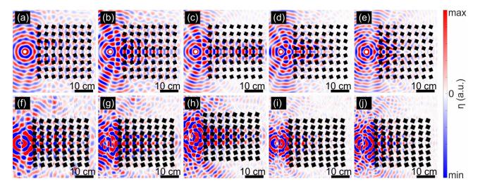
FIG. S3: Valley-Hall edge states: Experiments, and simulations. The water surface is perforated by  $8 \times 8$  square rigid inclusions. Numerics (top) and experiments (bottom) are shown at frequencies (a, f) 6.7 Hz, (b, g) 7 Hz, (c, h) 7.3 Hz, (d, i) 7.6 Hz and (e, j) 7.9 Hz.
