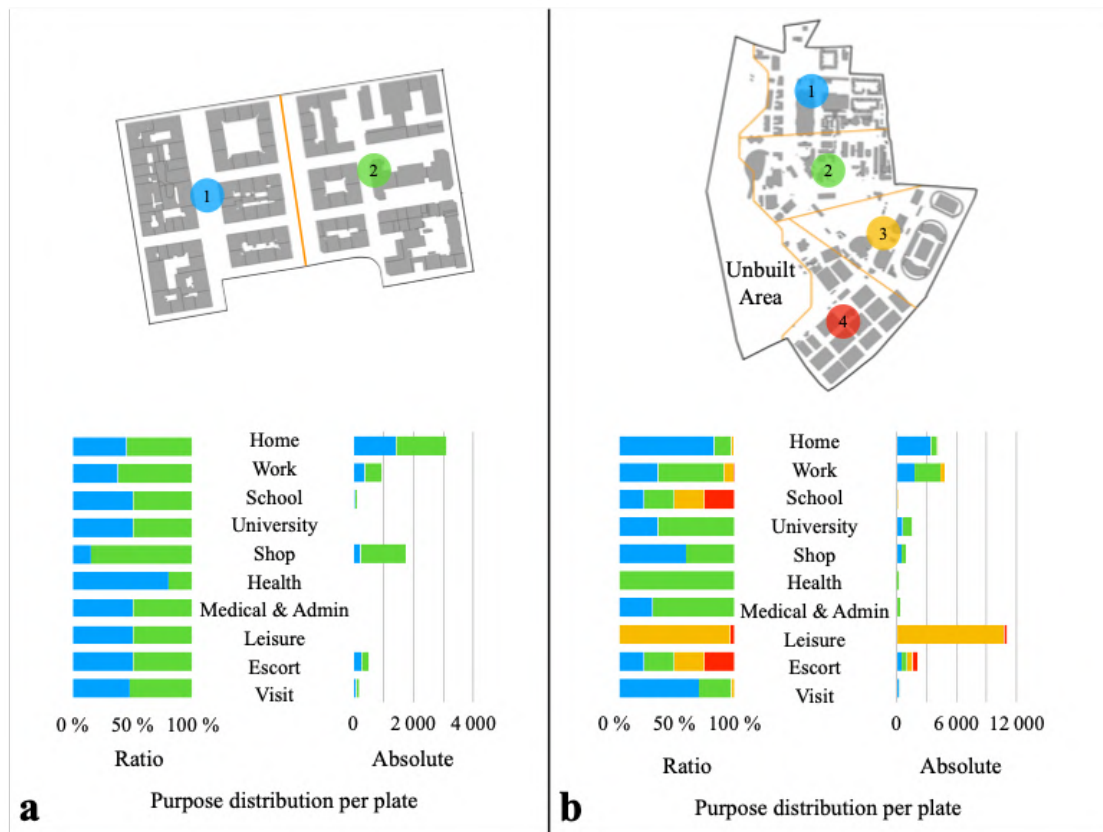
Figure 8: Results of the successive algorithms on two different areas: (a) “Saxe-Bossuet – a residential area, (b) “Tony Garnier” – a diverse area. Built is shown in dark gray, the orange line delimits FM-IRISes. The purpose distribution is also indicated as a ratio between the different FM-IRISes (left part of the graphs) and an absolute number of trips associated with the area (right part). The color code reflects different FM-IRISes.
