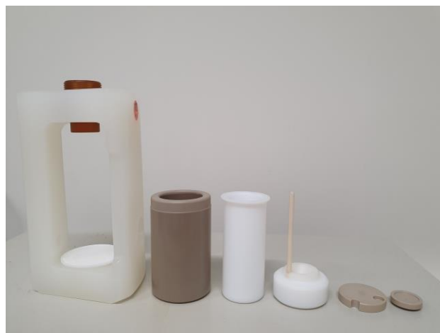
Figure 4: Hydrothermal microwave Polytetrafluoroethylene (PTFE) vessel
