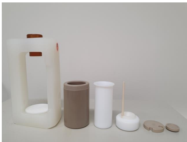
Figure 4: Hydrothermal microwave Polytetrafluoroethylene (PTFE) vessel
