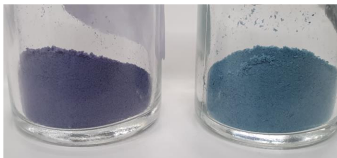
Figure 3: Left: Sepiolite+Tyrian purple after 140 °C in microwave for 25 min and drying for 24h at 150 °C. Right Sepiolite+Tyrian purple after 195 °C in microwave for 25 min and drying for 24h at 195°C
