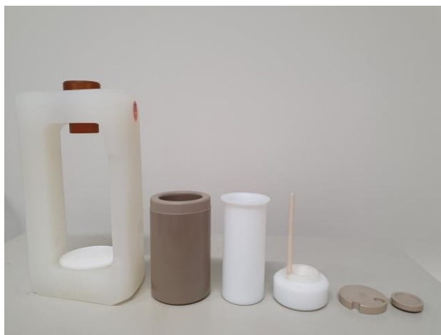
Figure 4: Hydrothermal microwave Polytetrafluoroethylene (PTFE) vessel
