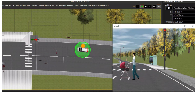
Fig. 5. Give way to pedestrians while preparing for the traffic light and entering the bus stop
