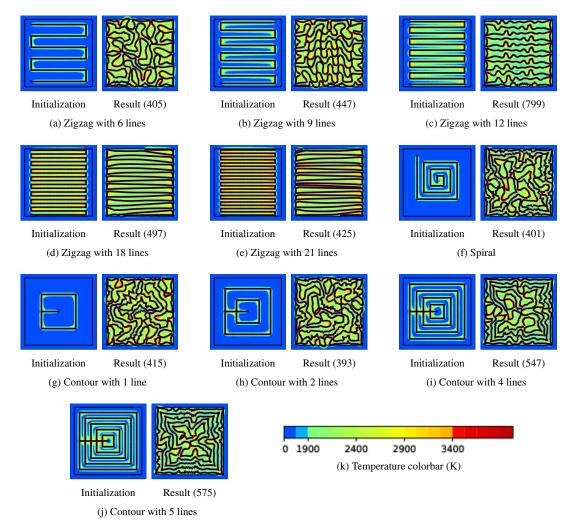
Figure 16: Path and maximum temperature  $(\max_{t \in (0,t_F)} y(t))$  during the building depending on the initialization (titanium)
