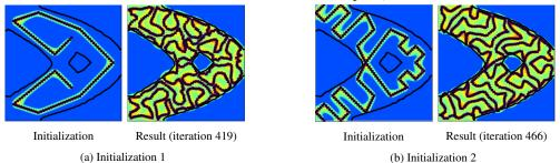
Figure 19: Path and maximum temperature  $(\max_{t \in (0,t_F)} y(t))$  during the building depending on the initialization for the one hole object (titanium)
