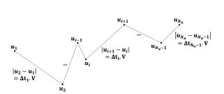
Figure 3: Front-tracking approach: fixed physical mesh and moving broken line path discretization
