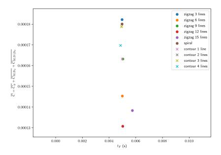
Figure 9: Constraint  $\overline{C} = \overline{C_{\phi}} + \overline{C_{\Sigma_S}} + \overline{C_{\Sigma \setminus \Sigma_S}}$  with respect to the final time  $t_F$  (s) for the final results (aluminium)
