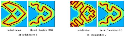
Figure 11: Path and maximum temperature  $(\max_{t \in (0,t_F)} y(t))$  during the building depending on the initialization for the one hole object (aluminium)
