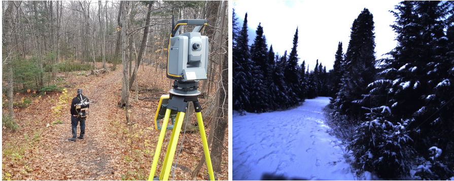
(a) Ground truth recording using the theodolite total station. (b) Snapshot from the center, backward-facing camera on the backpack sensor suite.
