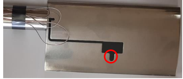
Figure 2: Foil section fitted with the e-telltale sensor. The sensitive moving part is shown by the red circle. The strain gauge is glued at the root (upper end on the picture) of the moving part.
