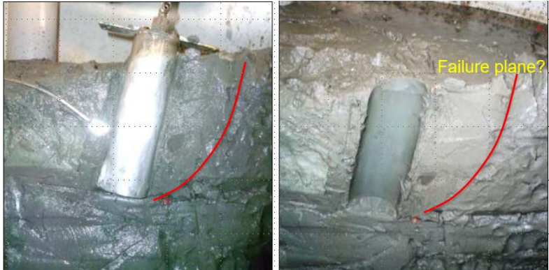
Figure 5: Backward rotation and failure plane (C9P2)
