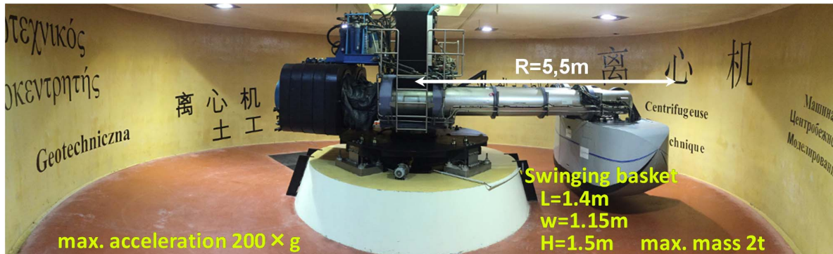
Fig.1 University Gustave Eiffel's geotechnical centrifuge
