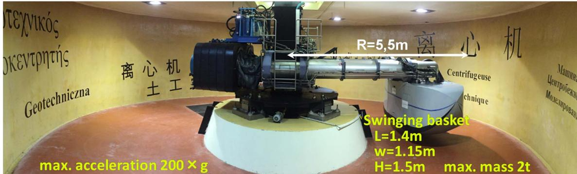
Fig.1 University Gustave Eiffel's geotechnical centrifuge
