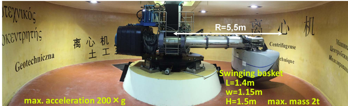
Fig.1 University Gustave Eiffel's geotechnical centrifuge
