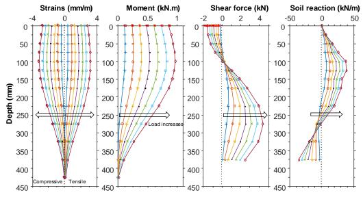
**Figure 2.** Profile of (a) the measured strains, (b) the bending moment, (c) the shear force and (d) the soil reaction (i.e., the distributed load) for seven horizontal loads (every 0.25 kN until 1.75 kN).
