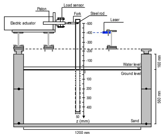
**Figure 1.** Schematic drawing of the horizontal loading system in the centrifuge at 100g.
