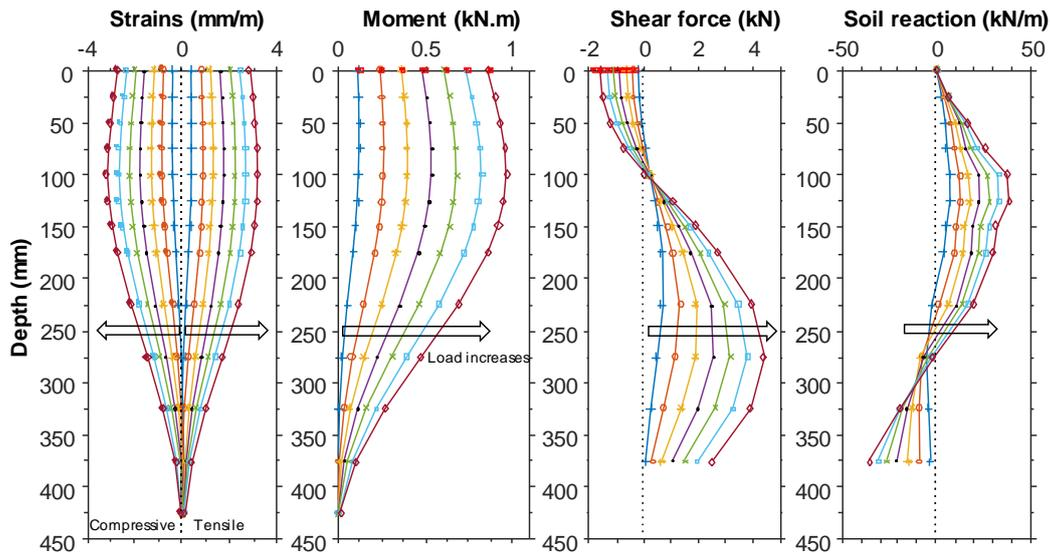
**Figure 2.** Profile of (a) the measured strains, (b) the bending moment, (c) the shear force and (d) the soil reaction (i.e., the distributed load) for seven horizontal loads (every 0.25 kN until 1.75 kN).
