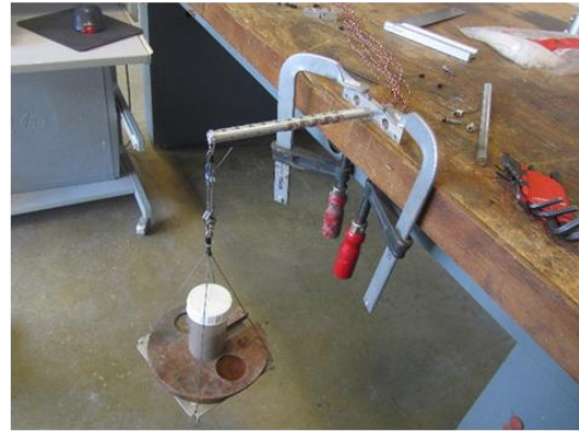
Figure 3. Model pile and calibration set-up.
