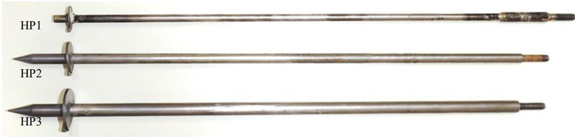
Figure 1. Helical pile models
