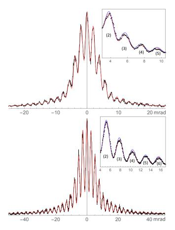
FIG. 2. Experimental diffraction spectra for beam velocities of  $26 \text{ ms}^{-1}$  (top) and  $19.1 \text{ ms}^{-1}$  (bottom) in black. The red curves are theoretical spectra with a single adjustable parameter  $(d_0)$ . The insets show individual diffraction orders. Black dots result from experimental spectra averaged over positive and negative diffraction orders. Red (blue) curves are calculated with CP (vdW) potentials.
