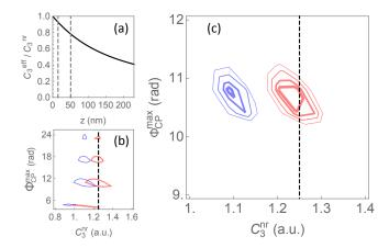
FIG. 3. (a):  $C_3^{\rm eff}/C_3^{\rm nr}$  as function of atom-surface distance. The two dashed lines represent the recorded atom-surface distance range. (b),(c):  $\chi^2_{min}+n\sigma$  [n=40 (b), n=1, 3, 6, 9 (c)] as functions of  $C_3^{\rm nr}$  and  $\Phi_{\rm CP}^{\rm max}$  at 26.2 ms<sup>-1</sup> for vdW (blue) and CP (red) potentials. The dashed line shows the theoretical value for  $C_3^{\rm nr}$ .
