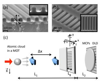
FIG. 1. SEM images of (a) a cleaved nanograting on a substrate and (b) a free standing membrane. (c) Experimental setup. An atomic cloud is periodically pushed by a laser (red arrow) from a MOT at a chosen velocity through a nanograting  $L_1=56$  cm away. A time-position detector is located  $L_2=308$  mm behind the nanograting. A light chopper (blue arrows) is available for accurate velocity measurement. A 6D piezo system controls the grating position.
