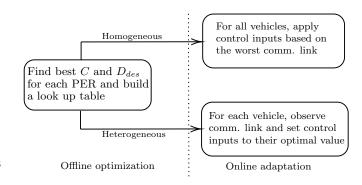
Fig. 3. Offline and online parameter election diagram.
