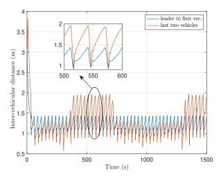
Fig. 5. Illustration of the average inter-vehicular distance for the first two and last two vehicles considering the Case 4 simulation.
