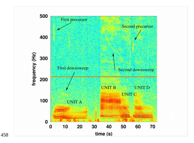
Figure 2. Time frequency representation of a SEP2 song recorded off Isla Chañaral, on February 2, 2017 (Fast Fourier transform, Blackman window of 65,536 points, overlapping 75%) using Octave software (Eaton, Bateman, and Hauberg, 2009). The line at 213 Hz is a constant electronic noise coming from the coupling between the hydrophone and the recording device. Units A, B, C, D are clearly visible as well as precursors and downsweeps belonging to the song.
