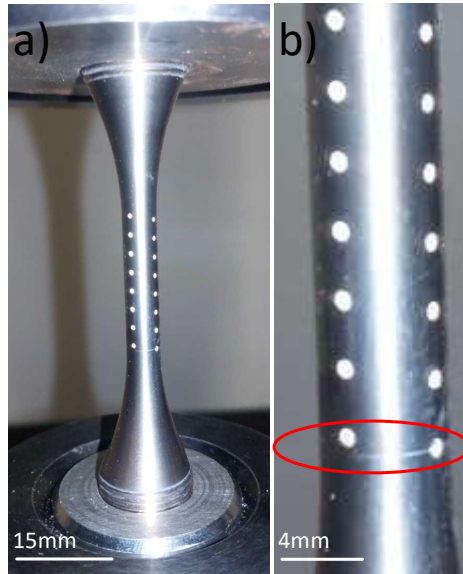
Fig. 6: a) Picture of the specimen containing 32 artificial defects, b) at higher magnification a crack that initiated from an artificial defect is surrounded in red.
