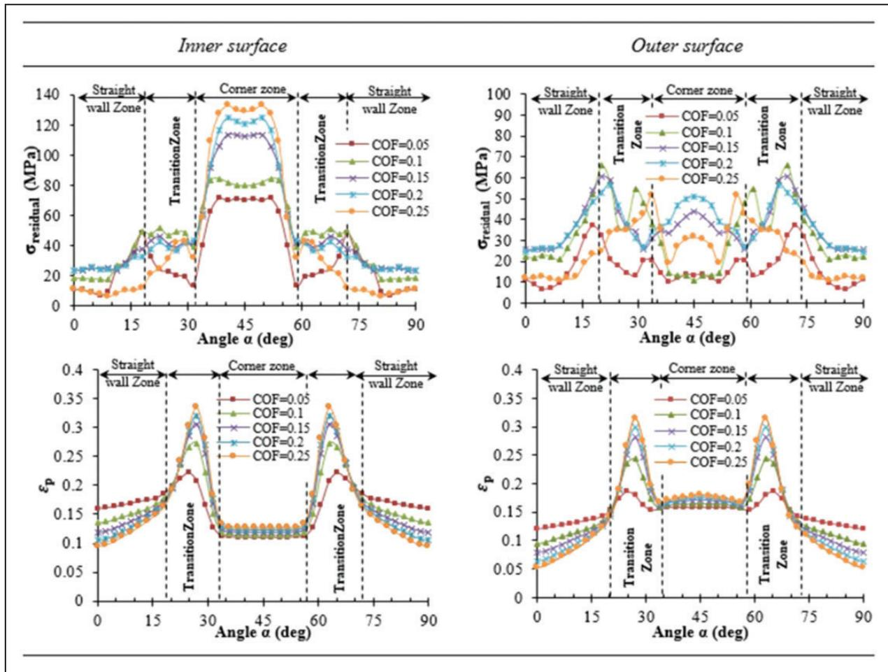
**Figure 11.** Distribution of residual stress ( $\sigma_{\text{residual}}$ ) and plastic strain ( $\epsilon_p$ ) in the tube cross-section after hydroforming process.
