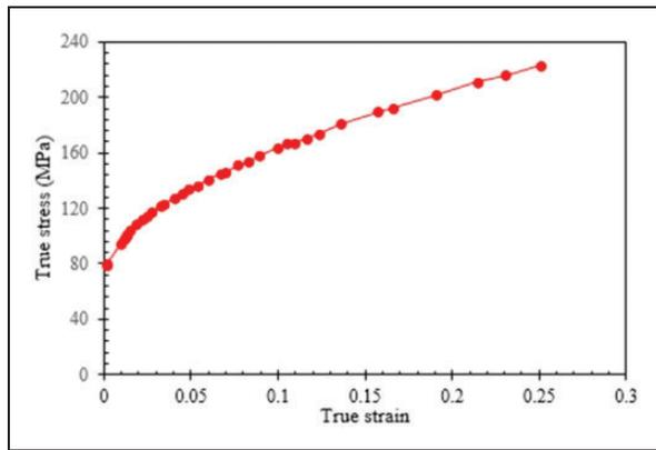
**Figure 1.** True stress–strain curve of deoxidized copper (Cu-DHP) at room temperature.
